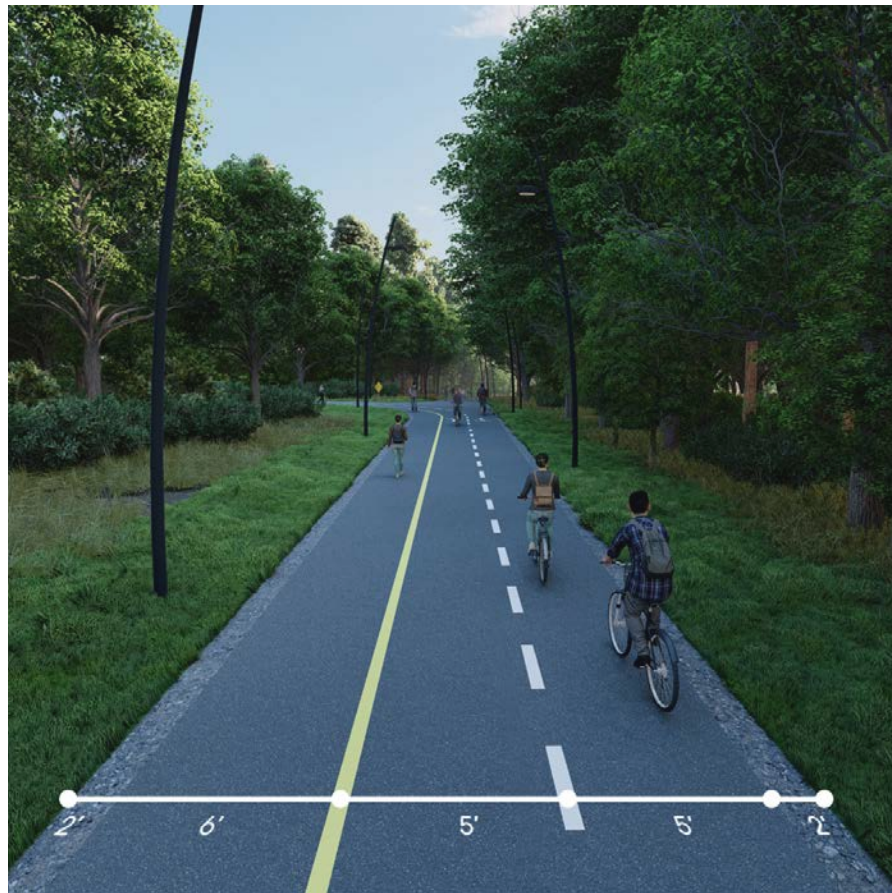
Preferred Bikeway Section - 16' Separated Use Path (10' Bike Path w/ 6' Pedestrian Path)
