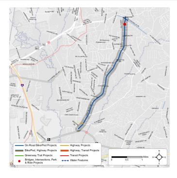
Construct westbound auxiliary lane along I-40 from NC 55 (Alston Ave) to NC 147. Planning and design for this project are in progress. Coordinate with I-5702 A.
